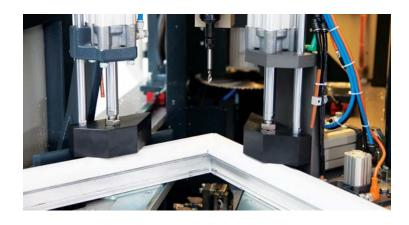
Single Line 2 Four Head Welding and CNC Corner Cleaning Machine
