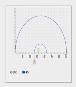
Max. Profile Cutting Height: 160 mm - +45 - 45 & 90 °
